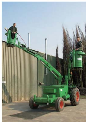
Self-built, self-driving pruning container system . Every container can be controlled individually so that the pruners can prune two rows in a single pass.
