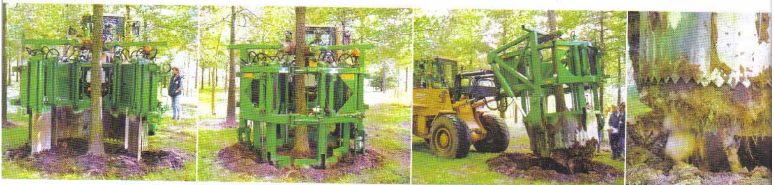
Lifting a Quercus palustris with the aid of a self-manufactured machine.
